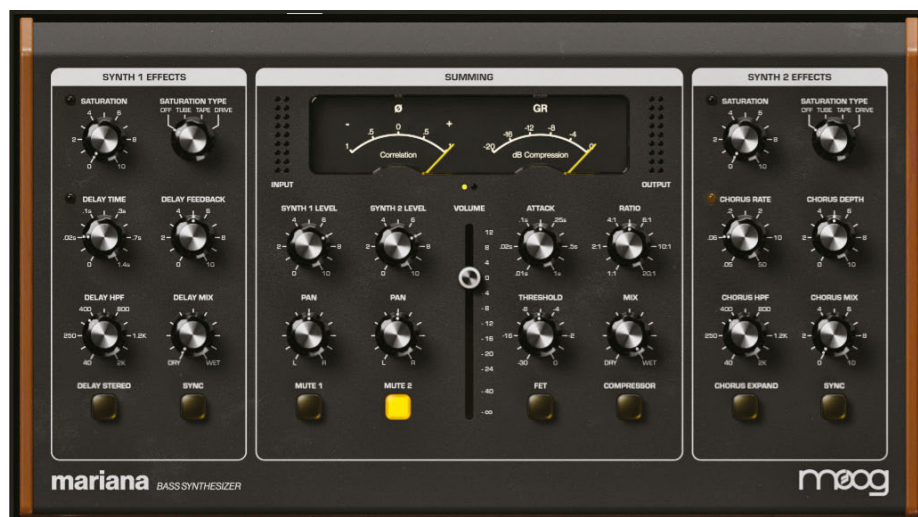
The Output page will sum the layers together, adding compression and effects too
